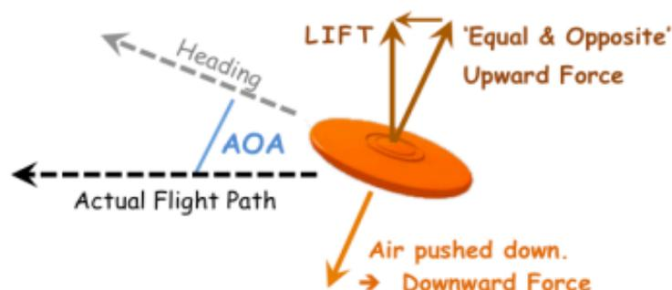
Figure 2: The key forces on a frisbee. [1]
